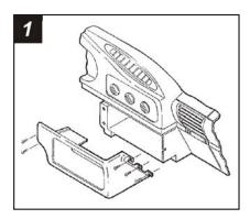
Disconnect the negative battery terminal to prevent an accidental short circuit. Remove (2) Phillips screws from the top of the driver's side knee bolster. Remove (2) 7mm screws from the bottom of the knee bolster. Open the glove box, remove (3) 7mm screws exposed on the right edge of the radio trim bezel and remove the bezel. Remove (2) 7mm screws securing the left side of the factory head unit and (1) 10mm nut securing the right. Slide the unit from the dash and disconnect the wiring.
